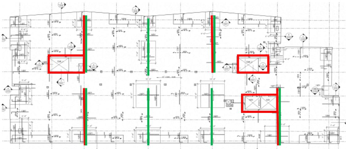
Figure 3: Typical Residential Floor Shear Wall Plan
